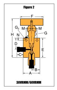
G<sub>1</sub> - Bracket mounting hole size Panel mounting drill size: 0:22" all valves.
