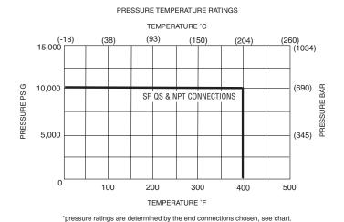
Maximum side connection inlet pressure 10,000 psi (690 bar)
