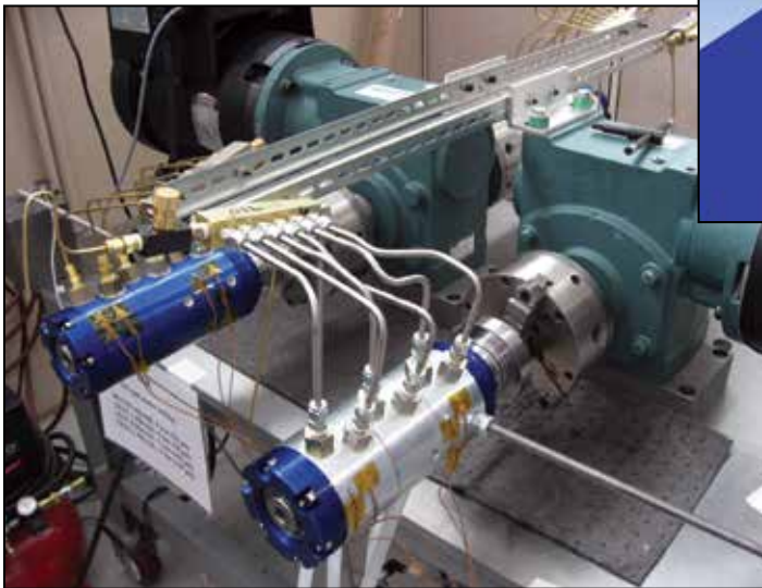
Deublin Multi-Passage unions testing fixture
