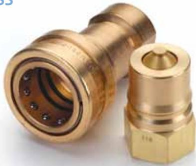
The HK brass is a general purpose industrial interchange coupling available in valved or non-valved designs, offered in brass for excellent corrosion resistance in rugged applications where stainless steel is unacceptable. Features a ball latch mechanism with automatic self-sealing poppet valves.
