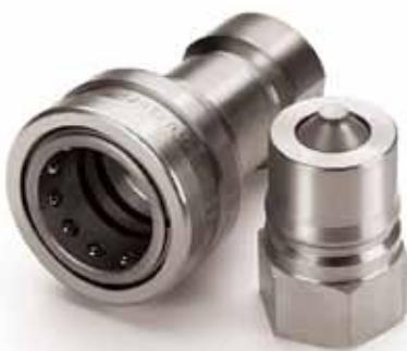
The HK stainless steel is a general purpose industrial interchange coupling available in valved or non-valved designs, offered in 303/316 grades of stainless steel for excellent corrosion resistance in rugged applications. Features a ball latch mechanism with automatic self-sealing poppet valves.
