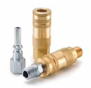
70 Series Pneumatic Couplers are interchangeable with Lincoln's "Long Stem" series couplings. Couplers have brass bodies and steel valves. Nipples are constructed of steel. Sleeve-Lok is an optional feature.
