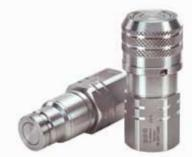
The Eaton MLFF Series stainless steel coupling is a flat face/dry break coupling used for hydraulic applications. The MLFF series interchanges with all ISO 16028 profiles. Due to its stainless steel design, it is corrosion resistant and can handle aggressive environments.
