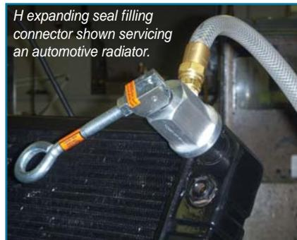
H expanding seal filling connector shown servicing an automotive radiator.
