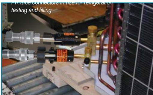
Designed to provide the sealing necessary for the greater sensitivity of today's demanding leak detection techniques.
