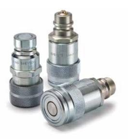
Parker Non-Spill Adapters were designed to accommodate the widespread use of several coupling types in mobile equipment. These adapters allow the user to adapt between poppet style, (ISO 7241-A), 6600 series couplings and non-spill type, (ISO 16028), FEM series couplings. They are useful where multiple hydraulic attachments are being utilized.
