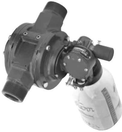
The Floco FRA Sampler is designed such that rotations of the Floco rotor drive a reduction gear train and, in turn, a disc valve. As the various ports in the discs align, flow is diverted from the process to an accumulator or from the accumulator to the receptacle bottle. The weight-activated full bottle shut-off trips a spring-loaded slide gate valve to stop the flow from the accumulator to the receptacle bottle.
