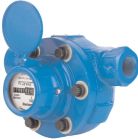
Like positive displacement meters, the Flotrac Meter is designed for mechanically measuring volumes of low-viscosity liquids flowing at high pressure. The Flotrac Meter employs the unique “constrained vortex” principle to provide an accurate measurement over a 10:1 range.
