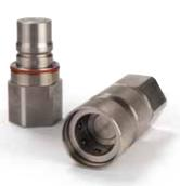
The NSE are dry-break couplings with flat face valves. The compact design makes it suitable for reduced spaces when high flow is needed. Coupling system with two-hand operation, i.e. both hands are required when connect/disconnect.
