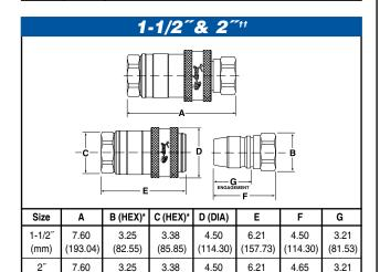
\*Hex dimensions are taken from flat of hex and not across corners. Hex may be substituted with round stock. Hex column would then indicate dimension taken across wrench flats. Decimal dimensions are ± .06 in. (1.5mm)
